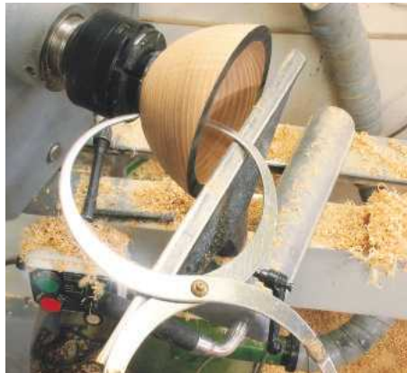
▲ Pic.5 Measuring is really important and there is no better way than using a simple set of figure-of-eight callipers. Always buy the biggest set you can, and for safety reasons, use them only when the lathe is switched off
